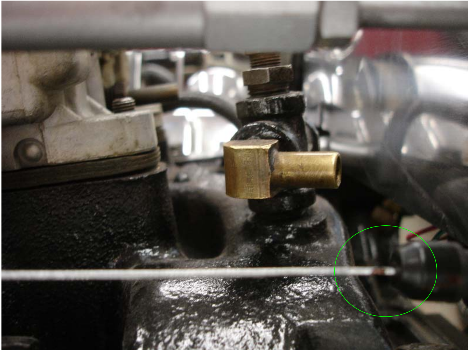
Position of TV cable at idle (see green circle)
