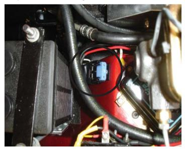
Because this alternator has an internal regulator, the original relic screwed on the inside fender can be bypassed. I chose to leave the old regulator it there so as not to change the car's appearance, but I "reassigned" the three original wires from the wiring harness so they now serve new functions.
